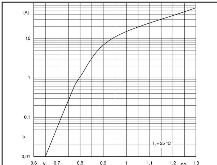
Fig. 1 Forward characteristic ( typical values )
