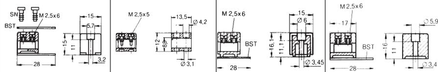
The MK 10/14 can be mounted using glue or with M 3 x 12 screws through the terminal point chamber.
