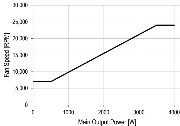
Figure 6. Fan speed versus main output power
