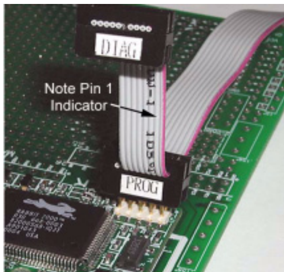
Figure 5. Connect Programming Cable to RCM2300
