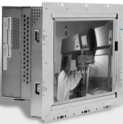
Open Frame Structure with IP-65 certified aluminum-front panel (optional)
