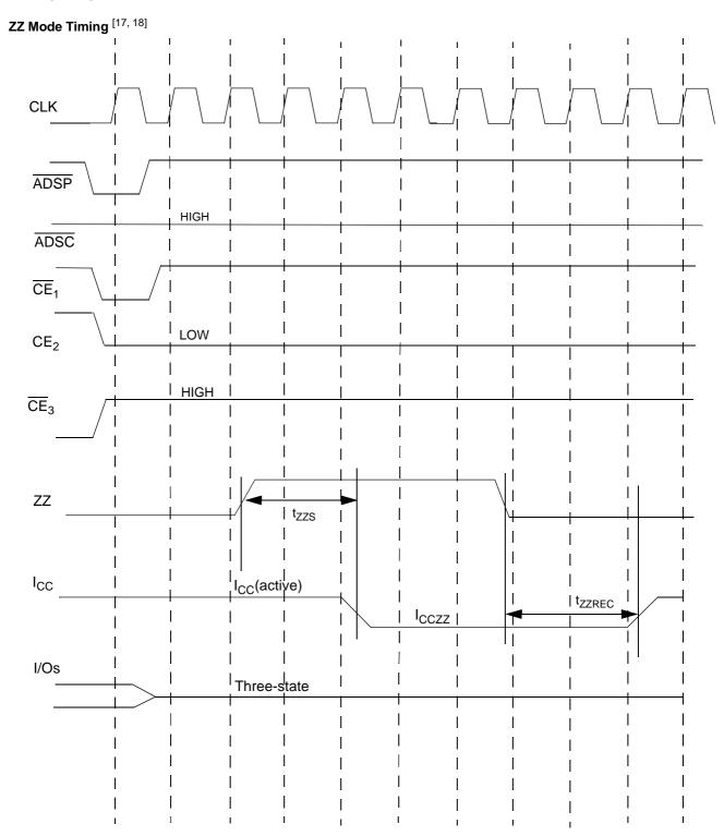
Device must be deselected when entering ZZ mode. See Cycle Description Table for all possible signal conditions to deselect the device. I/Os are in three-state when exiting ZZ sleep mode.
