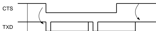
Figure 107. Transmitter Behavior when Operating with Hardware Handshaking
