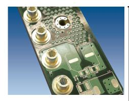
RADSERT<sup>™</sup>'s compact footprint design can deliver up to 120A of current to the board. The high current density and small surface area connection provides flexibility of board design. RADSERT<sup>™</sup> contacts are available in either press-fit or solder termination.
