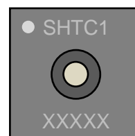
Figure 9 Laser marking on SHTC1, the top line with the pin-1 indicator and the sensor type, the bottom line with the 5-digit alphanumeric tracking code.
