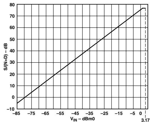
Figure 5b. S/(N+D) vs. V_{IN} (DAC @ 3 V) over Voiceband Bandwidth (300 Hz – 3.4 kHz)
