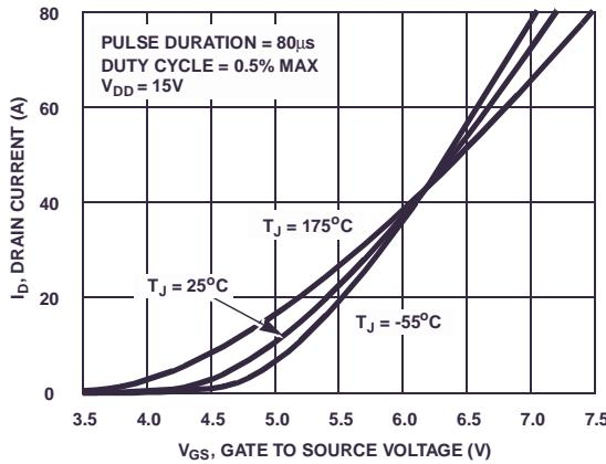
**Figure 7. Transfer Characteristics**
