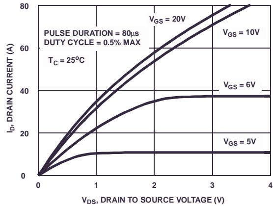
**Figure 8. Saturation Characteristics**
