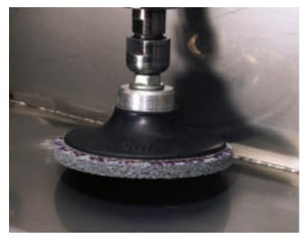
Scotch-Brite<sup>™</sup> Roloc<sup>™</sup> EXL Unitized Wheels are strong and efficient for edge deburring and finishing. They perform well in a variety of metal working applications and machined parts where close tolerances are important.
