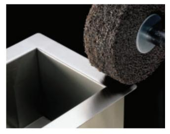
Multi-Finishing Wheels are highly conformable, soft wheels that create uniform and attractive final finishes on ferrous and non-ferrous metals. They are tough enough to finish edges and welds and soft enough to apply a final finish on large surfaces.
