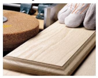
This wheel is a custom designed non-woven abrasive product for use on white wood sanding. An advantage of this wheel is the open construction and the use of garnet mineral, reducing the potential for part burning. The Scotch-Brite<sup>™</sup> Woodworking Wheel may be used in its straight form or shaped to various profiles.
