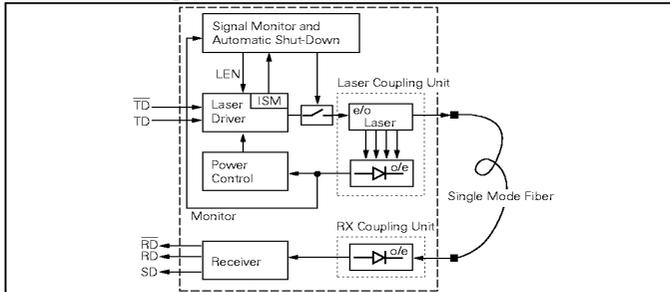
The receiver component converts the optical serial data into PECL compatible electrical data (RD and RDnot). The Signal Detect (SD, active high) shows whether optical data is present<sup>(1)</sup>.
