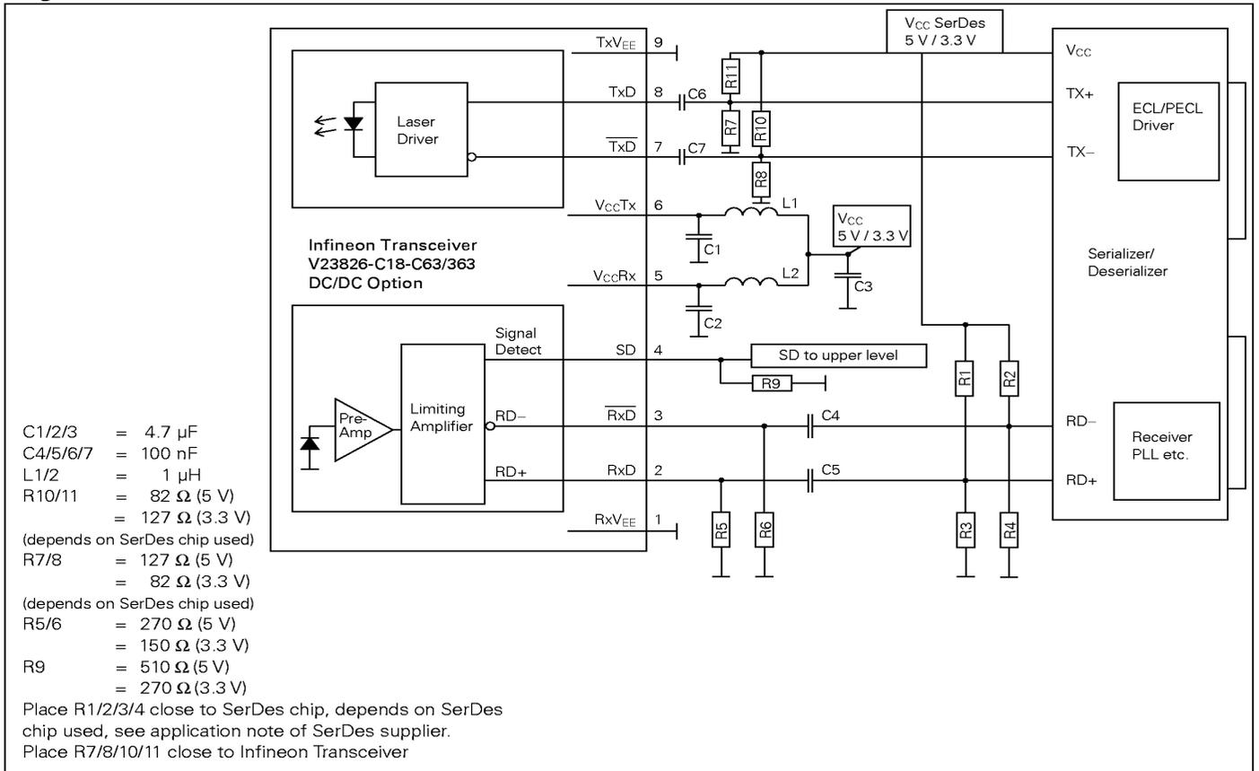
This Application Note assumes Fiber Optic Transceivers using 5 V power supply and SerDes Chips using 3.3 V power supply. It also assumes no self biasing at the receiver data inputs (RD+/RD-) of the SerDes chip (Refer to the manufacturer data sheet for other applications). 3.3 V-Transceivers can be directly connected to SerDes-Chips using standard PECL Termination network.
