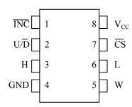
8-Pin DIP (300mil) 8-Pin SO (150mil) 8-Pin μSOP (118mil) 8-Pin Flip-Chip Package
