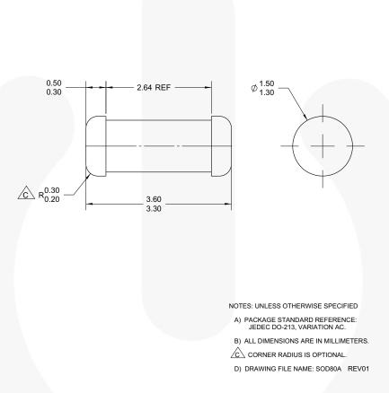
Figure 1. 2-TERMINAL, SOD-80, JEDEC DO-213AC, MINI-MELF
