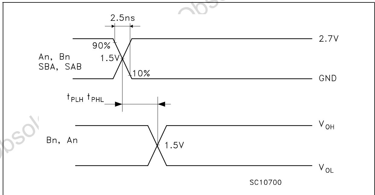
**Figure 7: Waveform - Output Enable And Disable Time (f=1MHz; 50% duty cycle)**
