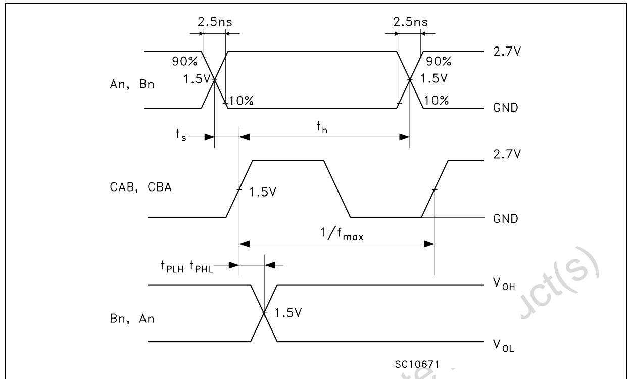
Figure 9: Waveform - Pulse Width (f=1MHz; 50% duty cycle)
