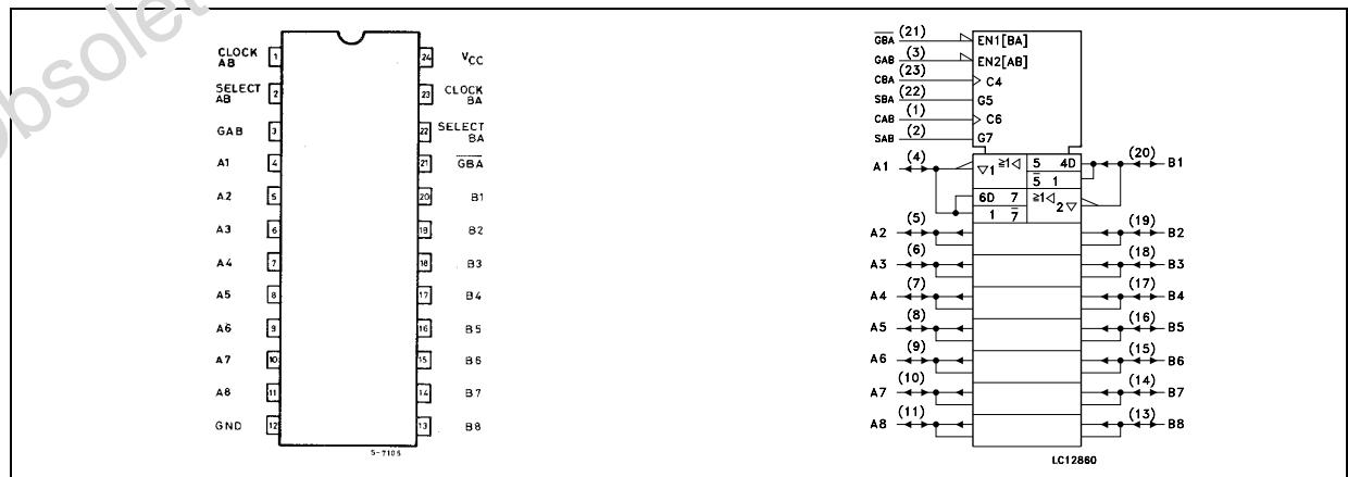
without using the internal D-type flip-flops by simultaneously enabling GAB or GBA. In this configuration each output reinforces its input. It has same speed performance at 3.3V than 5V AC/ACT family, combined with a lower power consumption.
